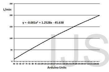
Fig.4 Polynomial function showing the relationship between the airflow and the Arduino units
