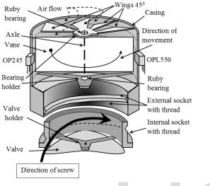
Fig. 2 Drawing of the turbine.
